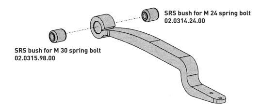
Once the spring bolt is correctly torqued after wheel alignment there is no need to re-torque the bolt after the first trip under loaded conditions.
