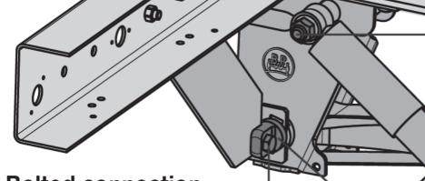
Bolted connection, gusset plate spring bolts:
